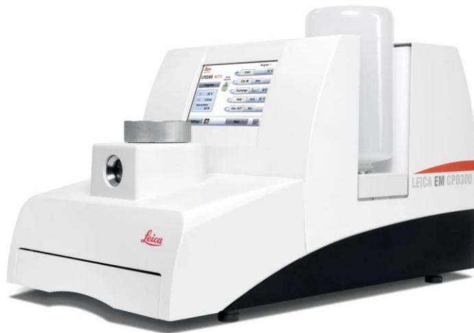
The Leica EM CPD300 is a fully automated critical point dryer designed for porous structure drying. It uses liquid carbon dioxide to dry samples without damaging their delicate structures.
