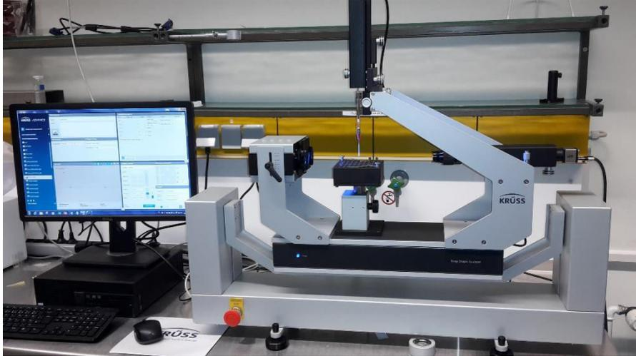
The KRÜSS model DSA25S Drop Shape Analyzer is a high-precision instrument designed for measuring of contact angle (static, advancing & receding, dynamic) of water or other liquids on solid surfaces in air or of air on surfaces underwater; measuring of surface free energy of solid surfaces; measuring of liquid sliding angle on solid surfaces
