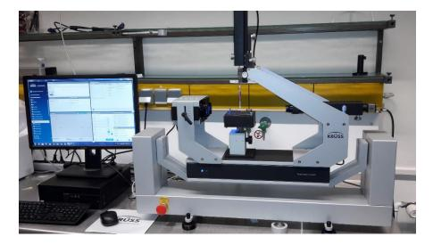
The KRÜSS model DSA25S Drop Shape Analyzer is a high-precision instrument designed formeasuring of contact angle (static, advancing & receding, dynamic) of water or other liquids on solid surfaces in air or of air on surfaces underwater; measuring of surface free energy of solid surfaces; measuring of liquid sliding angle on solid surfaces
