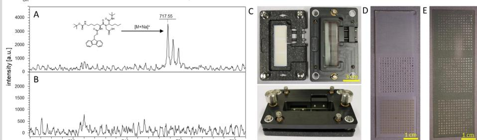
After photorelease into the droplets and addition of matrix, the array (D) can be copied to a MALDI substrate (ITO slide, E) by simple sandwiching (C) for mass spectrometry (detected product A and background B)
